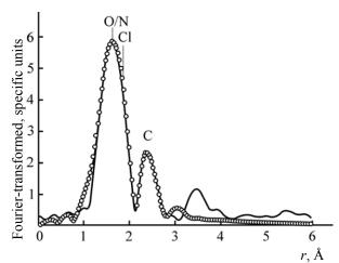
EXAFS-spectrum (CuK edge) of the [CuCl(HIpv)]·H<sub>2</sub>O (II) metal complex. (Solid line) experiment, (circles) calculation.
